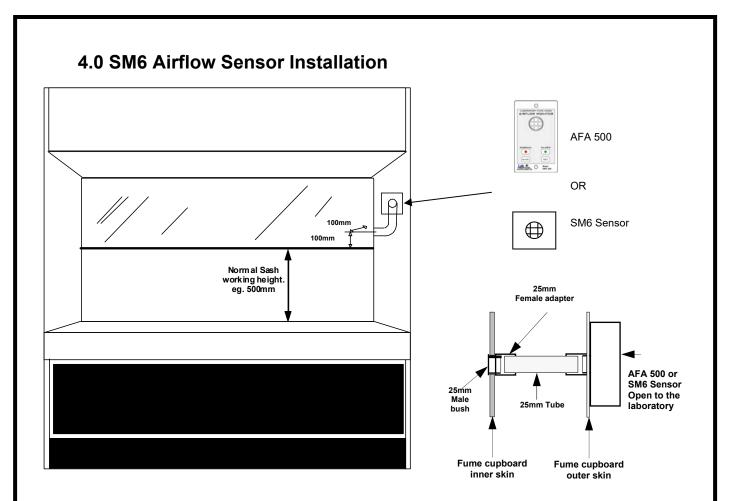
It is very important to position the AFA 500 or SM6 airflow sensor in the correct position to give long term stable reading of the face velocity. Please read the INSTALLATION NOTES below and if in doubt contact us for further advice.
