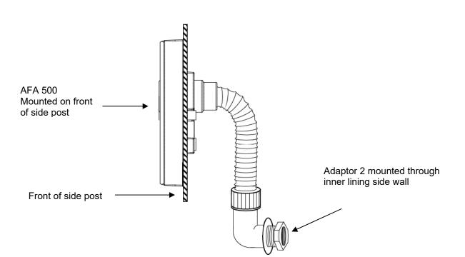
Loosen coupling Insert hose into coupling. Tighten coupling
