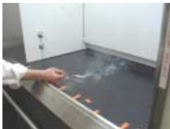
Figure 4 Low Volume Smoke Test
